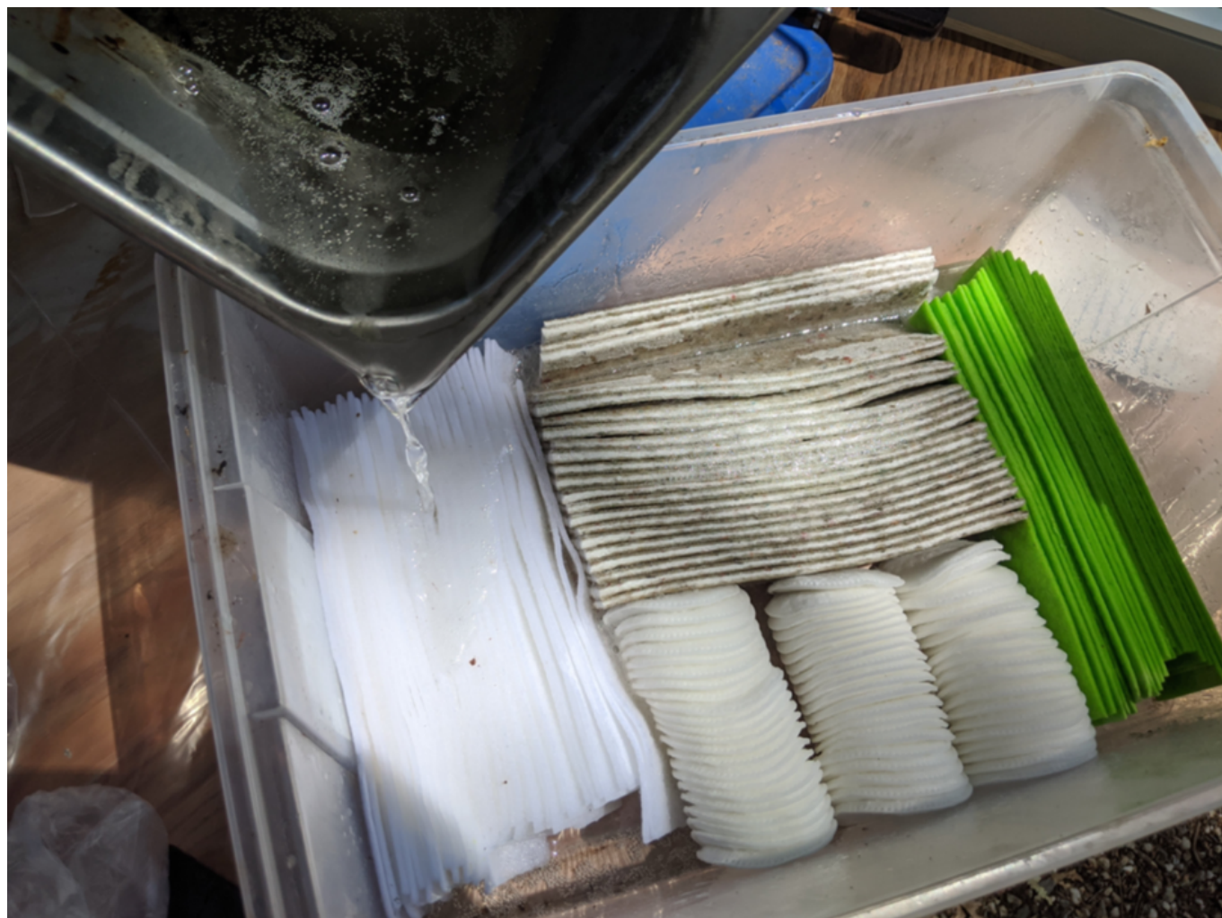
Fig. 3 I prepared the four matrices to be tested with the same batch of OA/gly solution at the 1:1 ratio. Tip: for full absorption, it's important to give any matrix enough room to expand.
