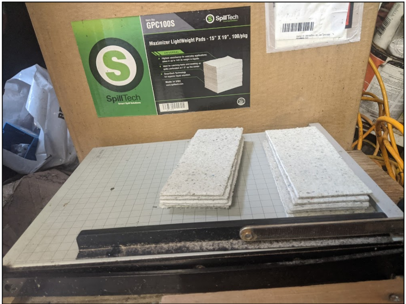
Fig. 11 A dedicated paper cutter with a built-in clamp allows for quick cutting of matrices. Here are ½-sponge equivalents of Maximizer lightweight pads, which are a readily-available alternative to Swedish sponges.
